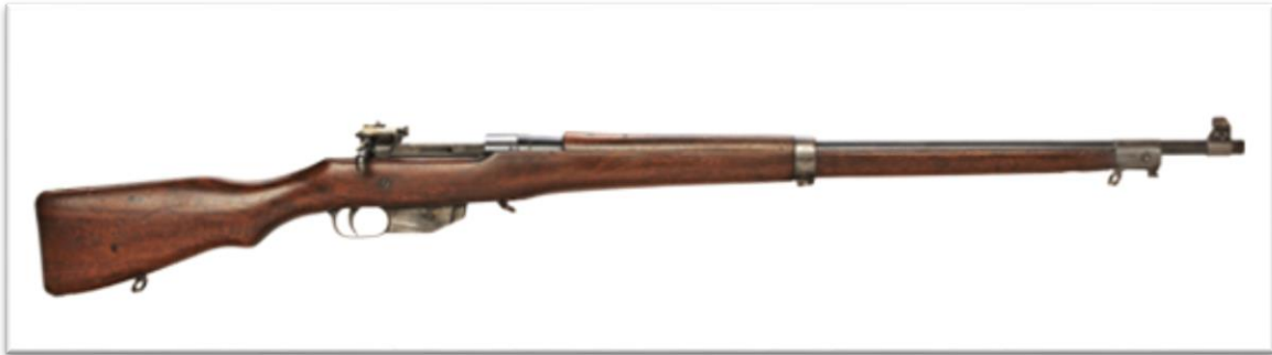
The Ross rifle is a straight-pull bolt action .303 inch-calibre rifle that was produced in Canada from 1903 until 1918.
